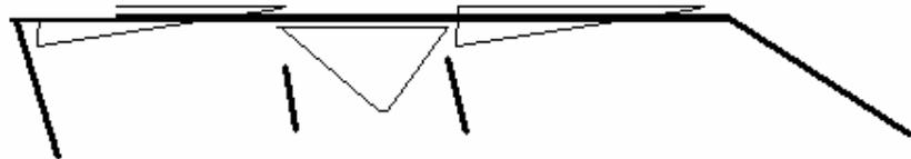
Figure 3, below, shows a rear view of the eyeglass frame. The 90 degree quartz prism can be either on the outside of the frame (Type -2A) or on the inside (Type-2B). Note that the point or apex of the prism points toward the user's forehead. If outside, it cannot touch or irritate the skin. If inside, then long nose pad legs must be used, and the frame is worn low on the nose, to prevent the prism's apex from touching the skin.
