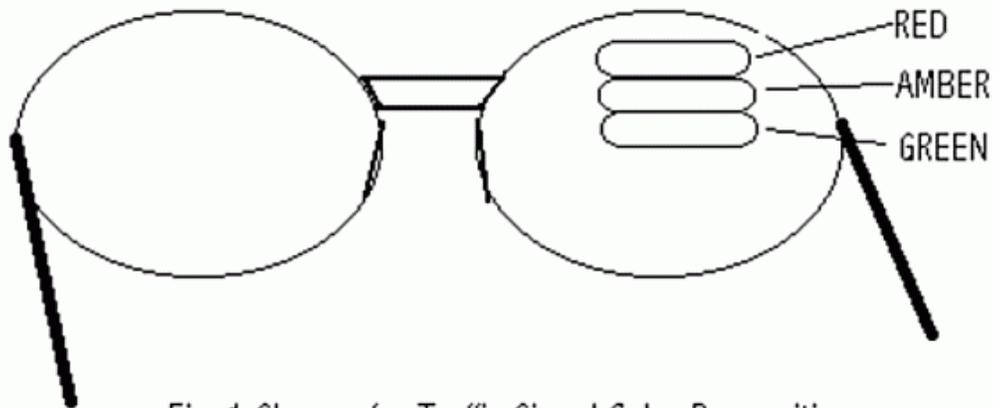
Fig. 1 Glasses for Traffic Signal Color Recognition
